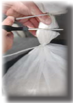
Photo 8- Apply second tie wrap and cut in- between tie wraps.
