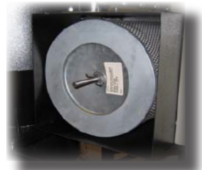
HEPA cover removed exposing cartridge
